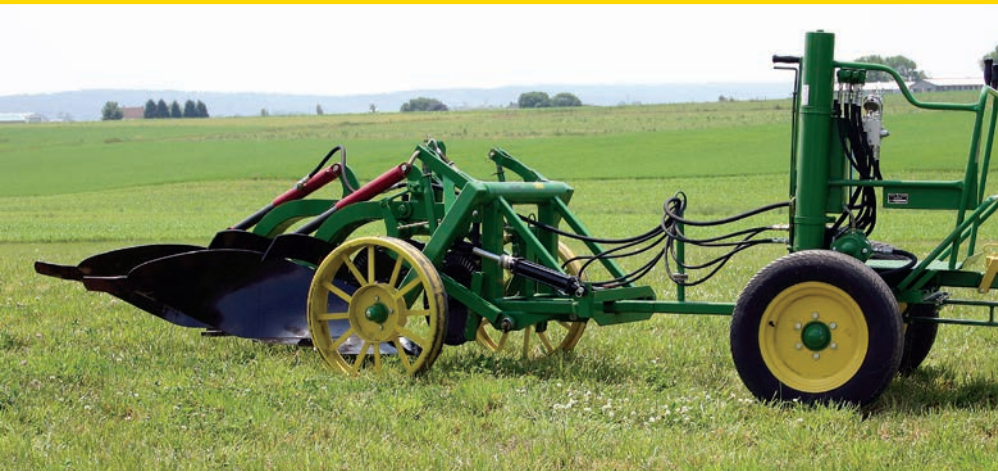
Showing #5 Keystone Sod Bottom with coulters & skimmers attached to 500 uni-frame & 631 forecart
