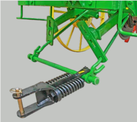
Full range draft adjustment with self-sliding spring hitch.
