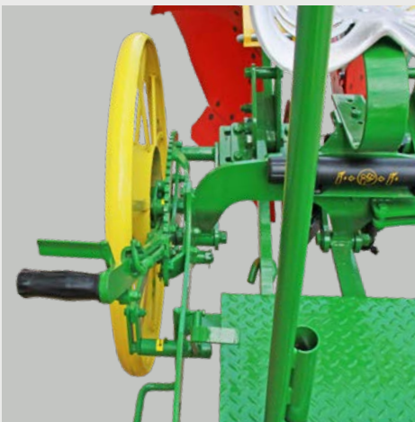
Foot activated wheel lift will fully raise bottom to a set position without using hand lever.
